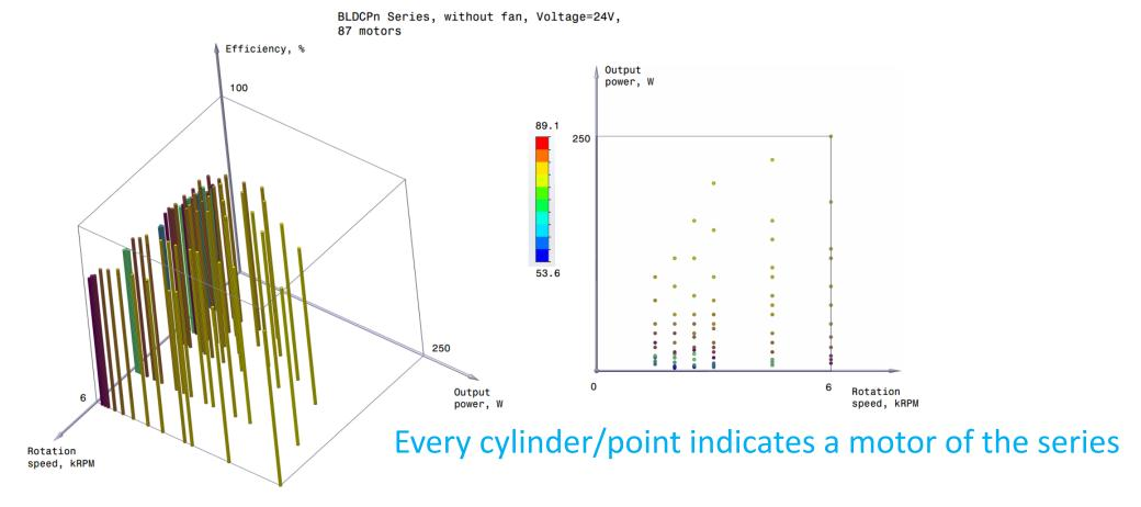
Efficiency chart for BLDCPn series without fan, 24V
