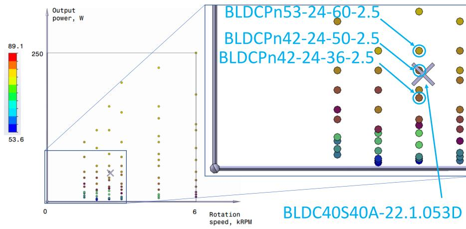
Efficiency chart for BLDCPn series without fan, 24V
