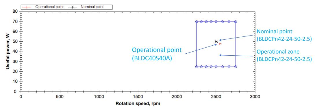
For every motor we identify an operational zone around the nominal point where acceptable efficiency and operating temperature are maintained
